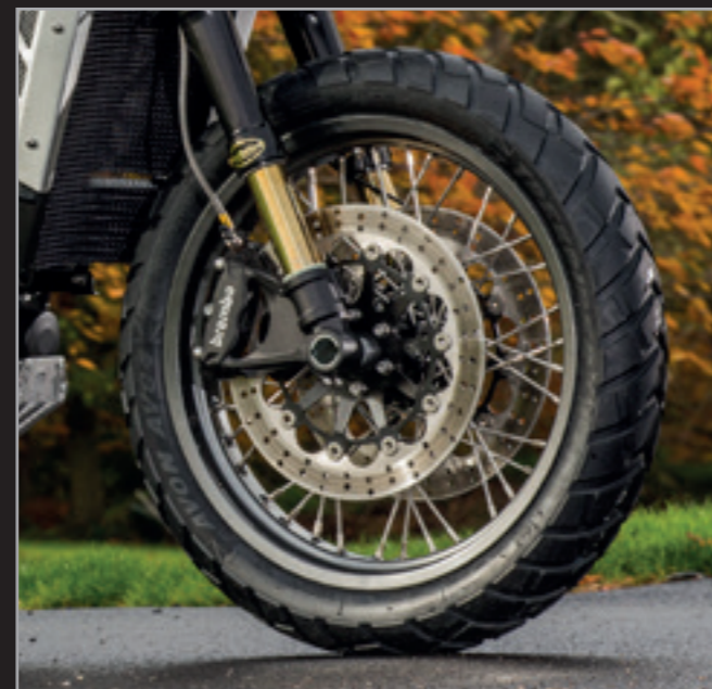
19" spoked wheel featuring Brembo, ABS, Roadholder and an Avon Trekriders tyre.
