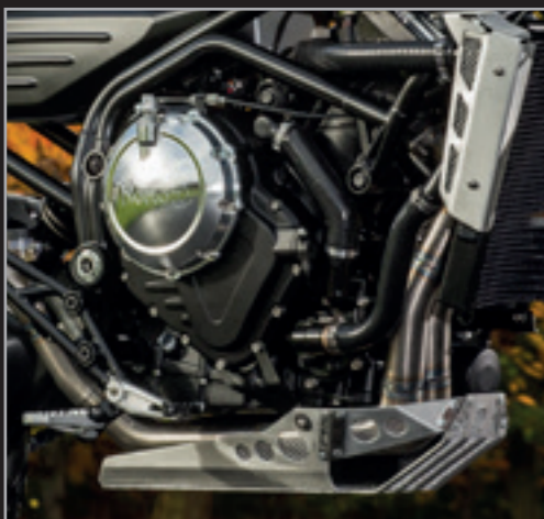
Strong-toothed foot-pegs with rigid bash tray protecting the beautifully styled 650 engine.
