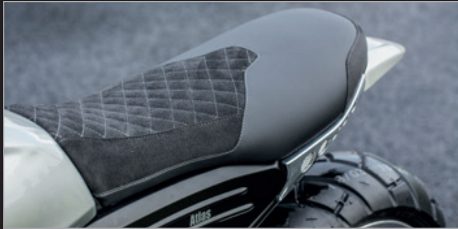
Nomad seat featuring Alcantara quilted panels with contrast stitching and embroidered Norton logo.
