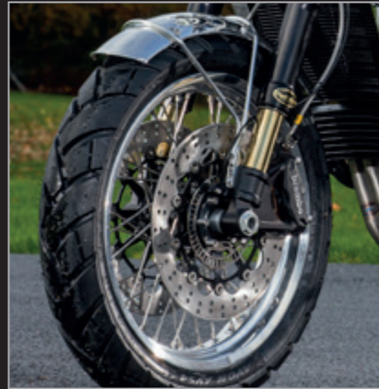
18" spoked wheel featuring Brembo, ABS, Roadholder, Avon Trekriders tyre along with sturdy polished aluminium mudguard.
